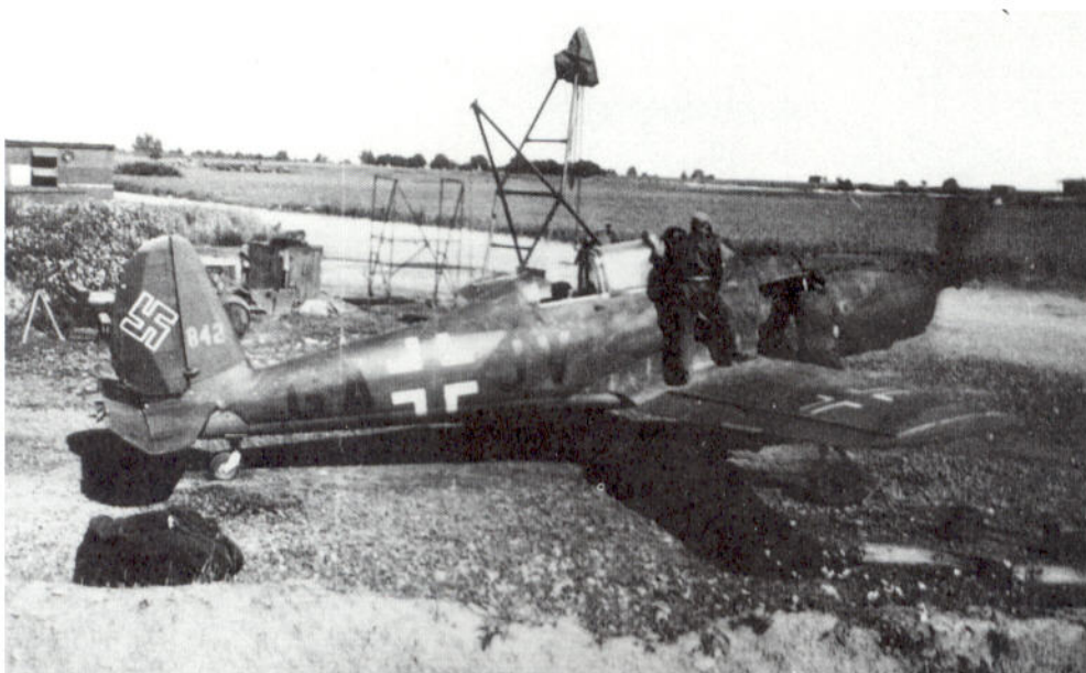
49: Trainer Arado Ar 96B, GA+JV, provides off-duty amusement for the ground crews of the US 324th Fighter Group. Despite the battered paintwork, the aircraft is probably in good condition, and the gantry in the background may mean that it has just had an engine change. Werk Nummer 842, is painted in yellow on the fin. Note the glossy finish of the letters compared to the camouflage. Stuttgart-Echterdingen June 1945
