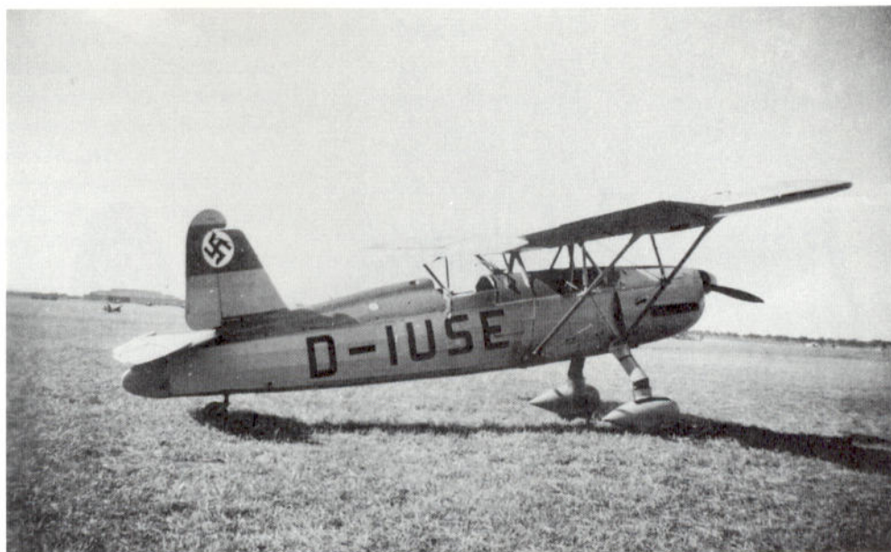
44: Starboard view of Arado Ar 76, D-IUSE, in use as a fighter trainer, probably in 1935-36. Note that the fuselage spine is painted, probably in blue. Location uncertain, but possibly Bernburg (AMC)
