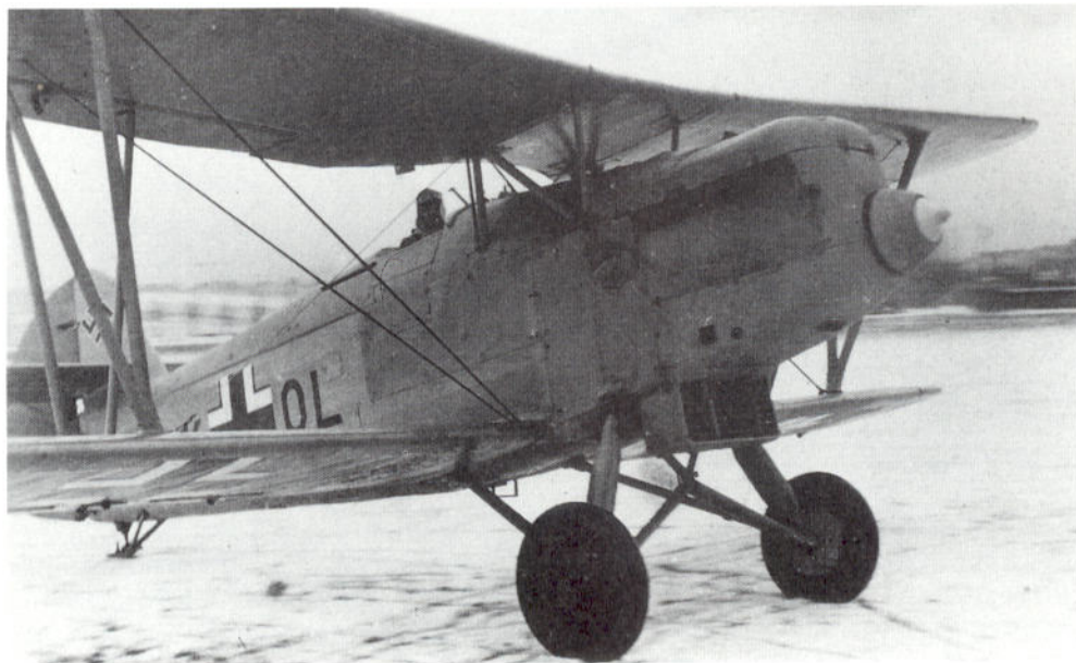
38: An elderly Arado Ar 65 fighter-trainer, coded ?K+OL, serving with FFS A/B 13 at Pilsen in Czechoslovakia taxiing out to the runway on a winters day, probably in late 1940. Finish is the typical well-worn RLM 02 Grau with a white spinner
